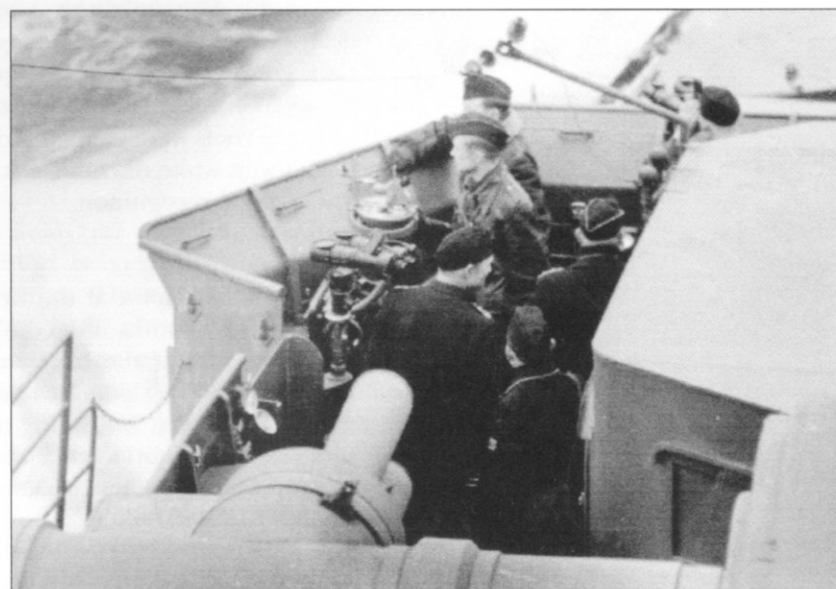
A view down into the bridge area of Prinz Eugen . This is the main open bridge, not the enclosed admiral's bridge up on the tower mast. This shot is taken from the roof of the forward command centre. The long tubular object in view at the base of the photograph is the housing for the rangefinder optics.
