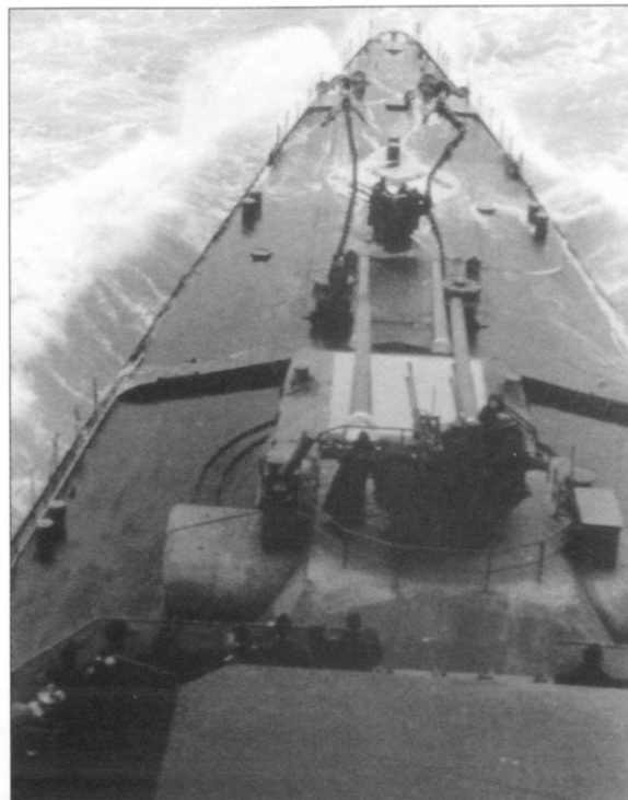
View over Prinz Eugen 's bow area, taken during the 'Channel Dash'. Note the quadruple-barrelled Flakvierling mounted on the forecastle and on the roof of turret 'Bruno'.
