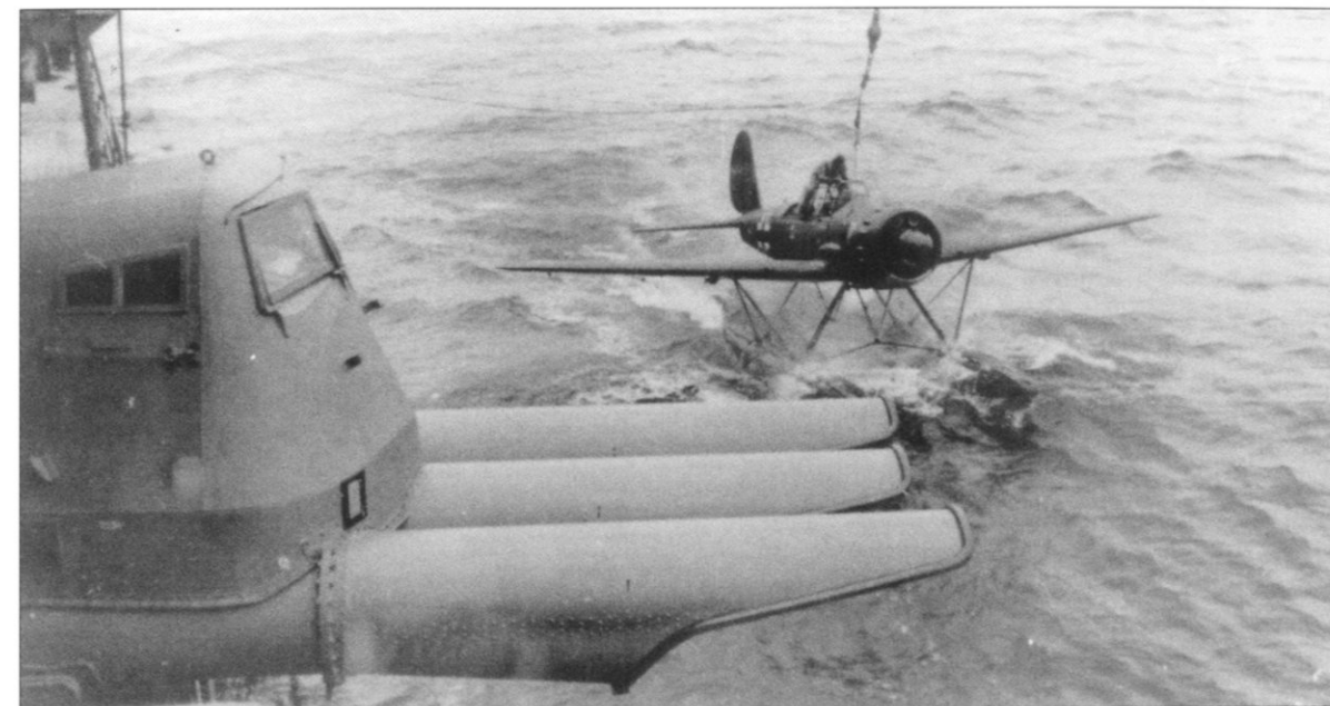
One of the triple torpedo tube sets on Prinz Eugen . Note the enclosed housing for the crew. The ship's Arado floatplane is taxiing alongside, about to be hoisted on board by the ship's crane.
