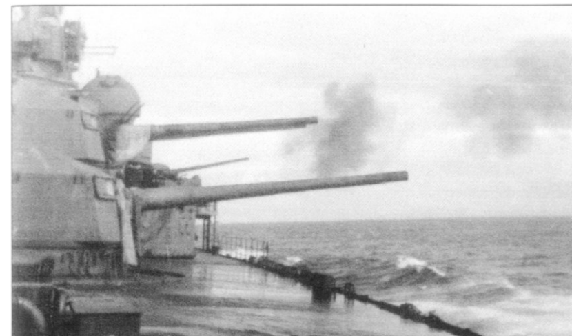
A view from astern with Prinz Eugen 's main armament trained out to starboard. The puffs of smoke are too small to be caused by firing of the main armament and seem to have come from the 10.5cm flak guns, the barrels of which are visible in the space between the gun barrels of turrets 'Caesar' and 'Dora'.
