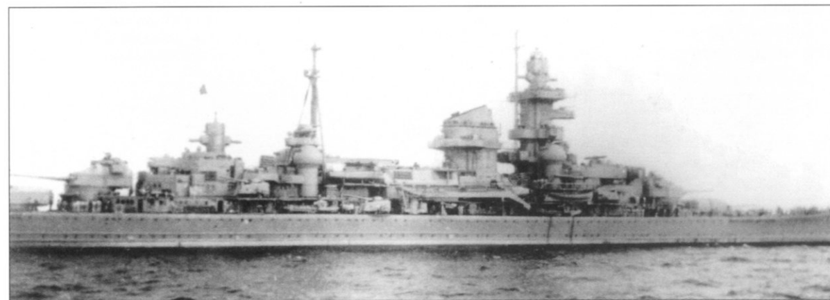
A snapshot of Admiral Hipper taken from a U-boat whilst on training exercises in the Baltic. This shot gives a good view of her midships section. Note the flak gun platform fitted on the roof of turret 'Caesar' and the extensive modification to the rangefinder housing on the foretop when compared with earlier photographs.
